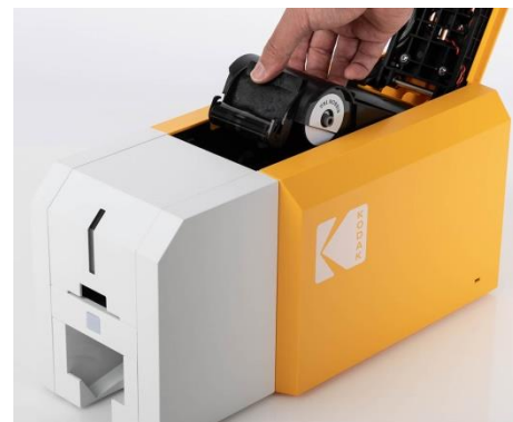
Figure 11 Installing the ribbon cartridge
