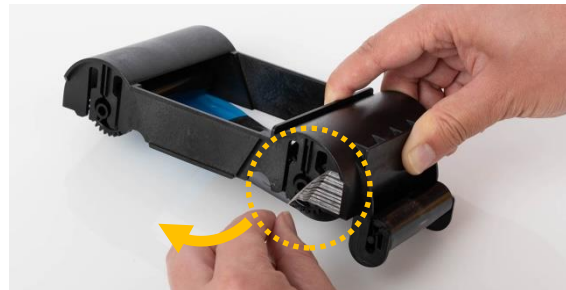
Figure 10 Peel off the ribbon position tape
