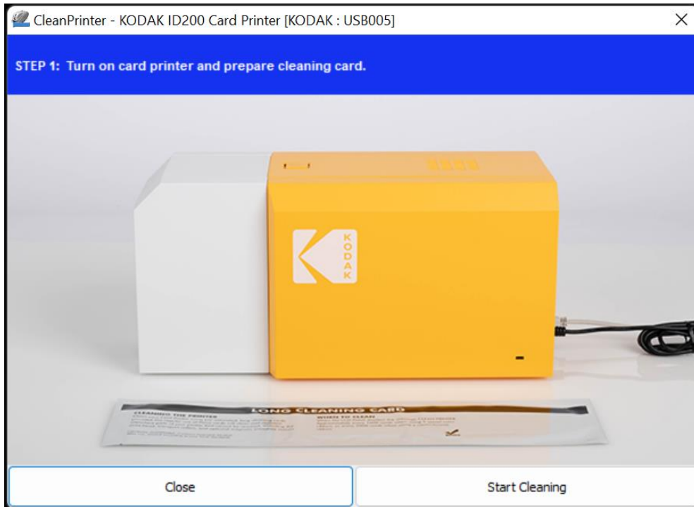
Figure 57 Printer cleaning Step 1
