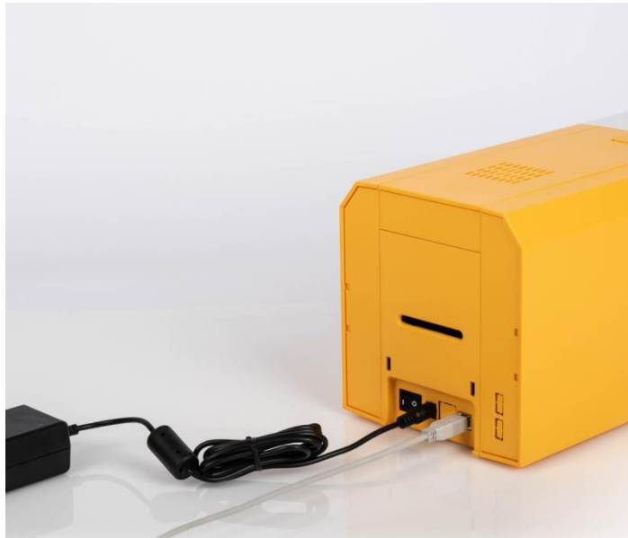
Figure 6 KODAK ID200S Connection of power and USB cable
