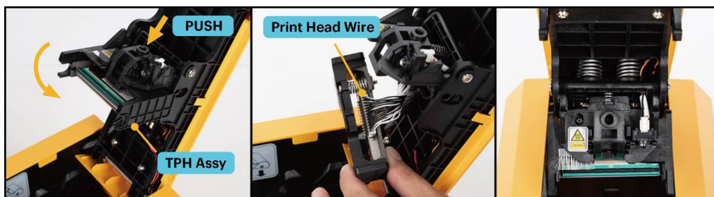
Figure 60 Print head replacement
