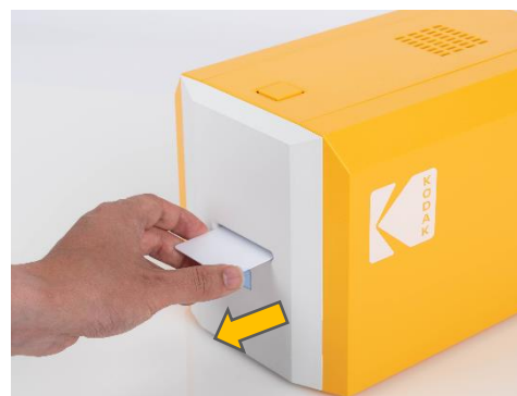
Figure 15 Unloading the card
