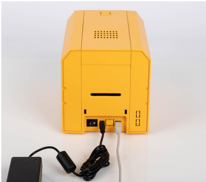
Figure 6 KODAK ID100S Connection of power and USB cables
