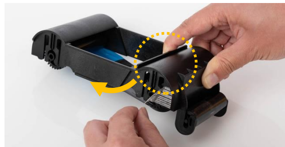
Figure 10 Peeling the ribbon position tape
