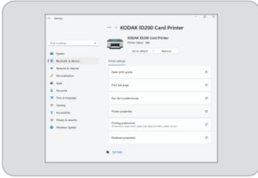
※ For Windows 7/ 8, access Windows Control Panel and select Device and Printers. Right click “KODAK ID200 Card Printer” and select “Print Properties”.
